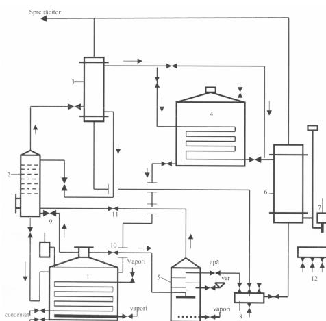
**(54) Intermittent-duty plant for direct distillation of wines with high content of sulphur dioxide**
